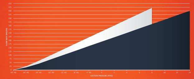
FX12 MSCFD - 2200 RPM, Pd-100, 2.28 Gear FX12 MSCFD - 2200 RPM, Pd-150, 1.74 Gear
