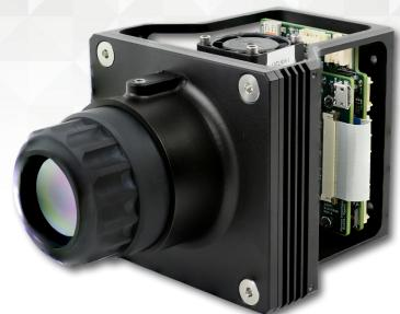
**Vayu HD Details:** With true 1920x1200 (Full HD) resolution from an uncooled VOx microbolometer array, the Vayu HD is the highest-resolution LWIR camera on the market. At just 450 and 520 grams (25 and 50mm lens versions) and compact enough to fit in the palm of your hand, the Vayu HD sets a new standard for superior image quality and resolution in a SWaP optimized package.
